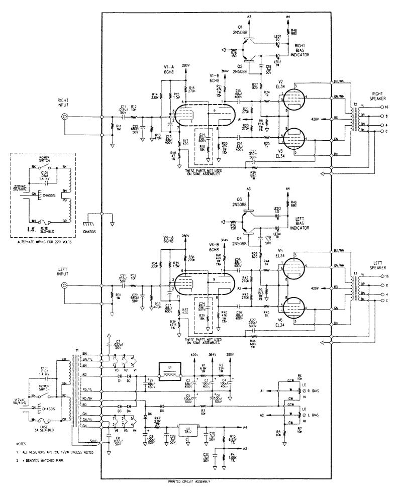
Output Paralleling your ST70 II for 70W mono operation:
